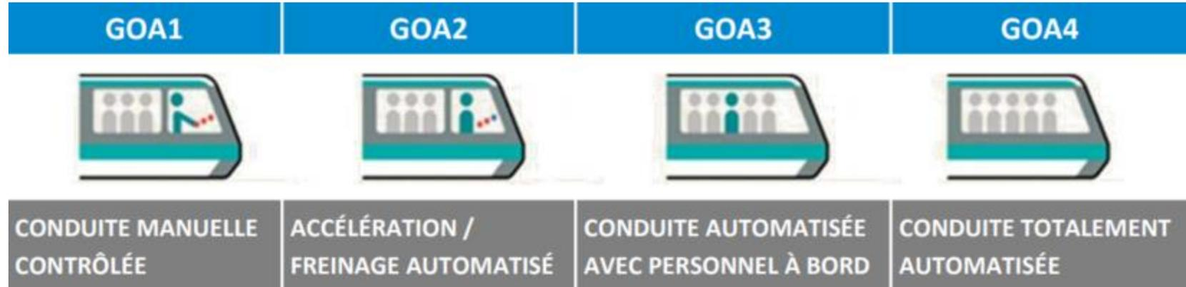
GoA2 is an intermediate level of automation that provides the service of acceleration and deceleration. It is supervised by the **Automatic Train Protection** system (ATP). The conductor is always in charge of the exchanges with passengers, door control and unexpected situations.
